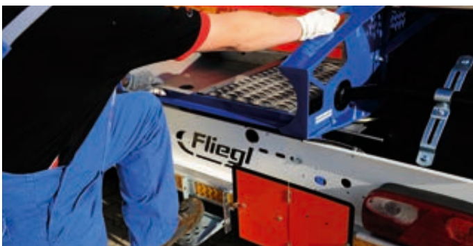
Fliegl provide hand-holds and steps for improved working safety.
