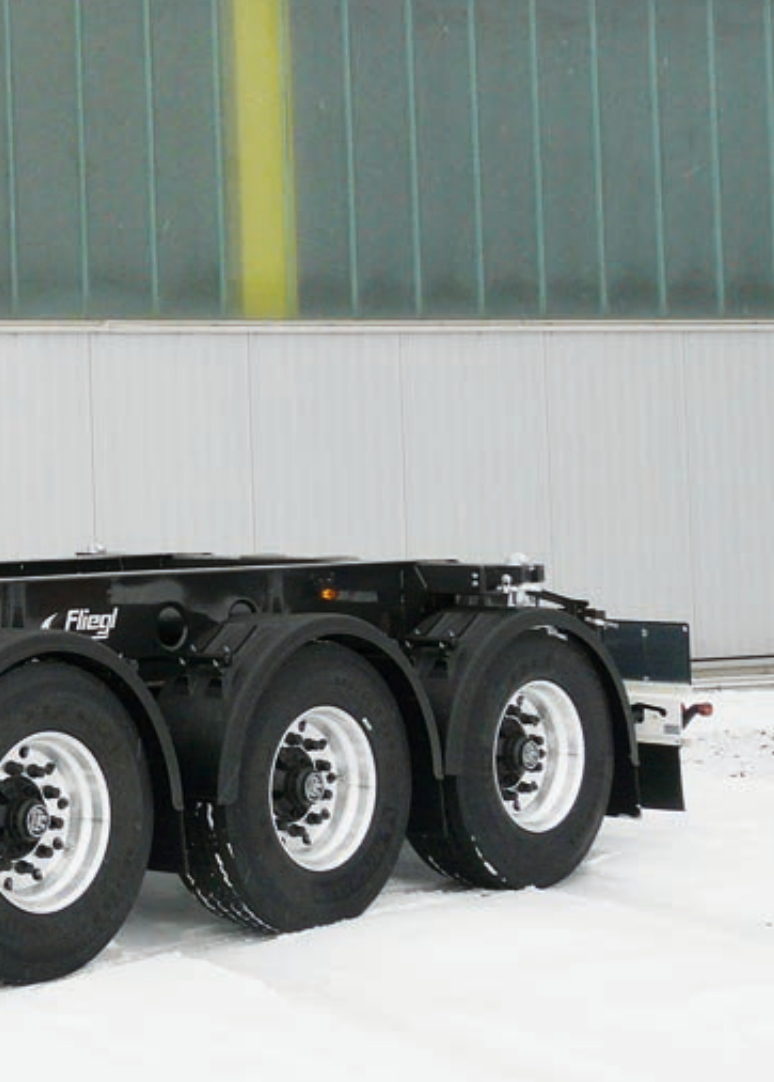
Chemical chassis Light for 20 foot containers and 7.82 series tank containers
