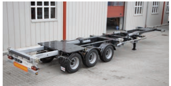
Optimum load distribution and coupling load through the middle attachment on a 20 foot container.
