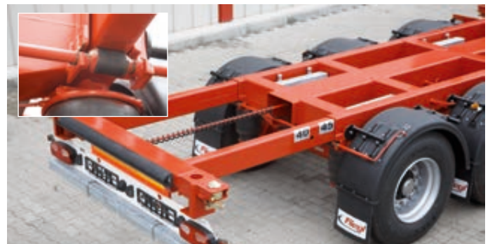
Manual, roller bearing rear extension booms: Robust, smooth running, disturbance free
