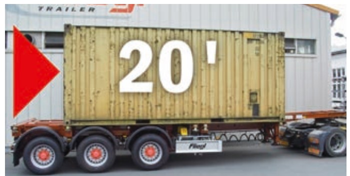
Vario chassis V3 with sliding device for 20 foot containers
