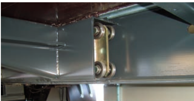
Tandem roller bearings for rear extension booms
