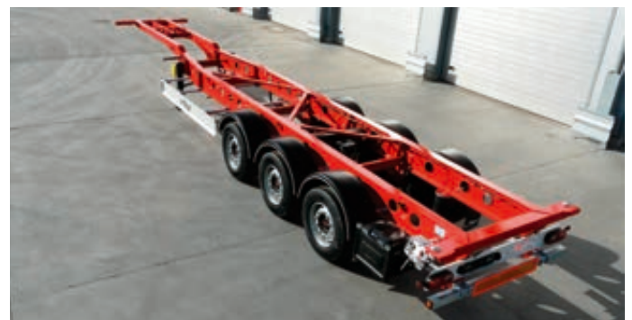
40 or 45 foot chassis in light configuration from 3450 kg
