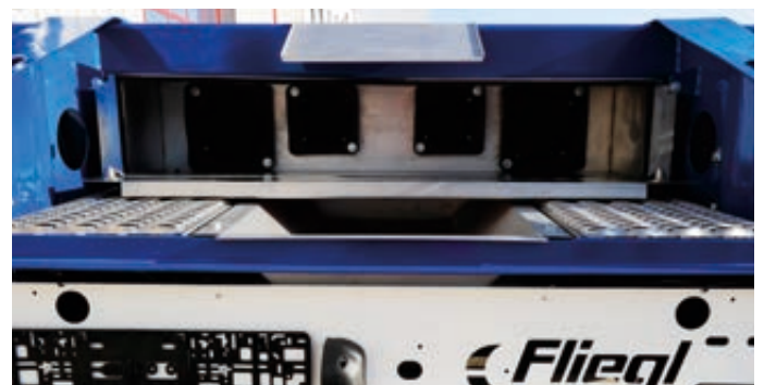
Stainless steel hose boxes with drain for hoses
