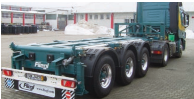
Vario dump chassis for 20 and 30 foot containers
