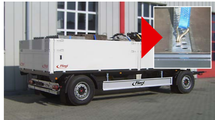
Pivot plate construction material trailer – total weight 18 tonnes with traverse perforated sections for variable fastening of lashing straps, fitted as standard.
