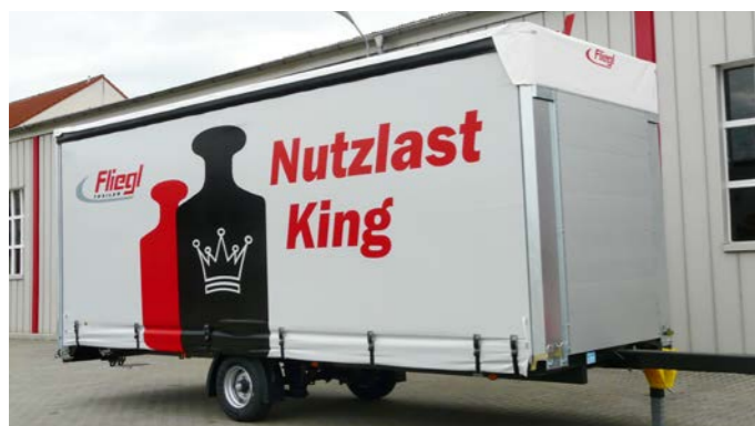
Fliegl's payload king, a platform trailer with a sliding curtain body that weighs less than 2 tonnes. When coupled to a 7.5 tonne HGV it makes up a train that is below the 12 tonne toll limit.
