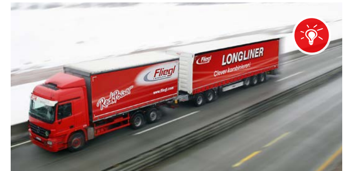
The Road Train consists of an HGV (two or three axle tractor unit) with a fixed or interchangeable body, a Dolly and a three axle semi-trailer (Standard, Mega or Jumbo).
