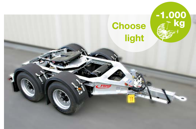
The Fliegl Dolly is available as Standard and Mega. The steerable version is the lightest on the German market – with an unladen weight reduction of up to 1000 kg and a payload capacity increase of up to 1000 kg compared to models from other manufacturers. Instead of a steering axle, hydraulic cylinders in the tow bar steer the Dolly round the corners. The mechanism is technically uncomplicated, not susceptible to faults and low in wear and tear and maintenance.
