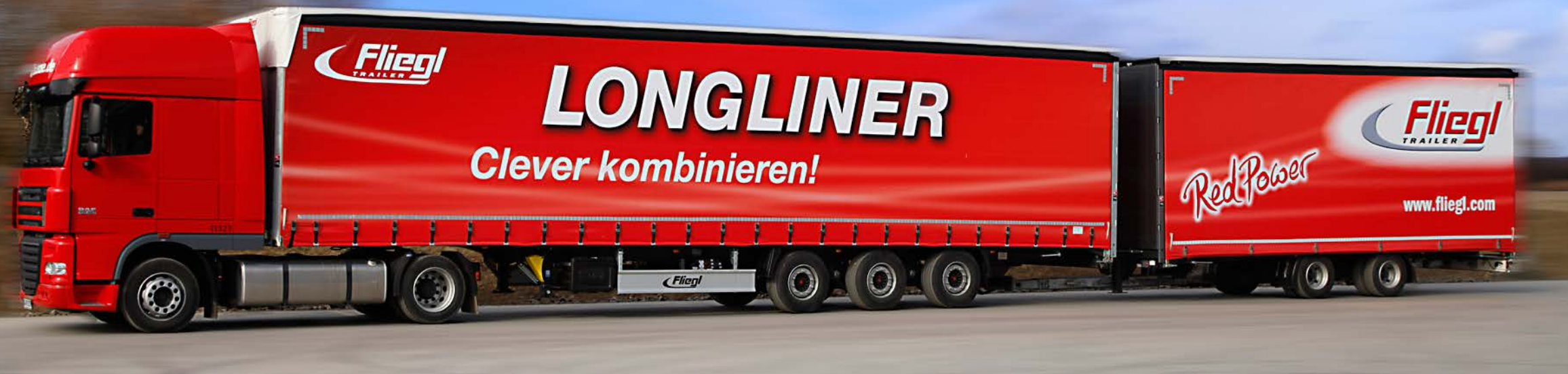
The Super Train consists of a Standard, Mega or Jumbo semi-trailer and a tandem trailer.
