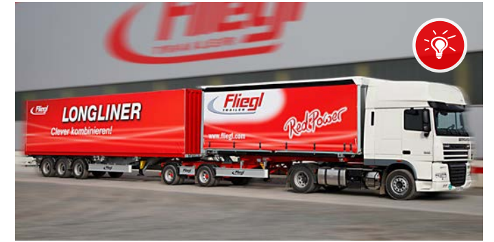
The Combi Train consists of a special semi-trailer with a movable axle unit for rear-end loading and unloading of the trailer (a container chassis is also possible). The trailer, like the tractor unit, has a fifth wheel coupling, on which a second semi-trailer (Standard or Jumbo) can be towed.
