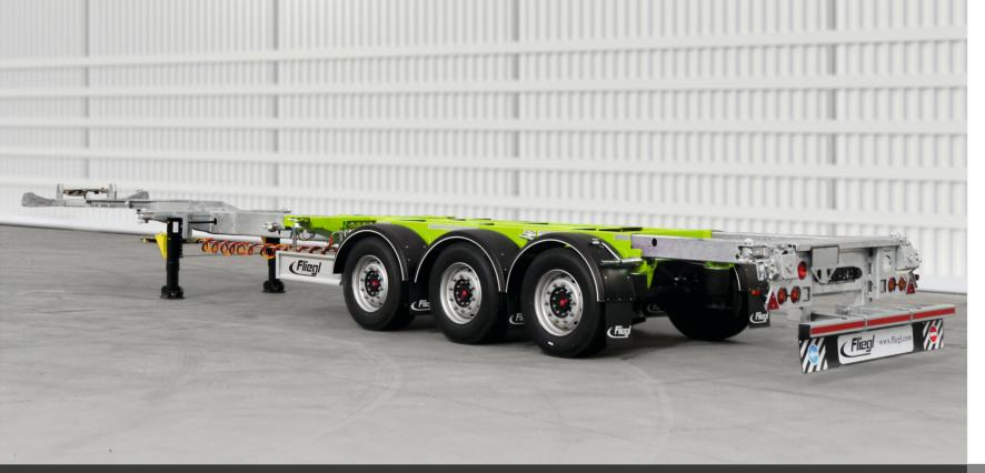
**3-axle container semitrailer Vario** SDS 380 V3+ with front extension New Generation
