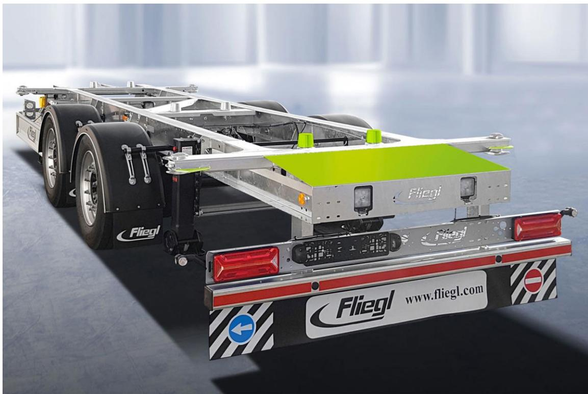
The TWP 180 Standard offers mounting options for three different swap body dimensions: the container locks on stable booms are suitable for containers with lengths of 7.15, 7.45 and 7.82 metres. Fliegl equips its tandem swap body trailers with three pairs of removable guide rollers; the Swap Guard swap body positioners before and behind each container lock facilitate positioning of the containers and prevent collision damage. The front stop can be adjusted longitudinally and folded down.
