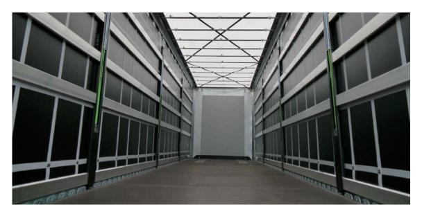
To maintain full loading height when loading from the side, Fliegl uses its special **non-elastic roof bar** made of high-strength aluminium.
